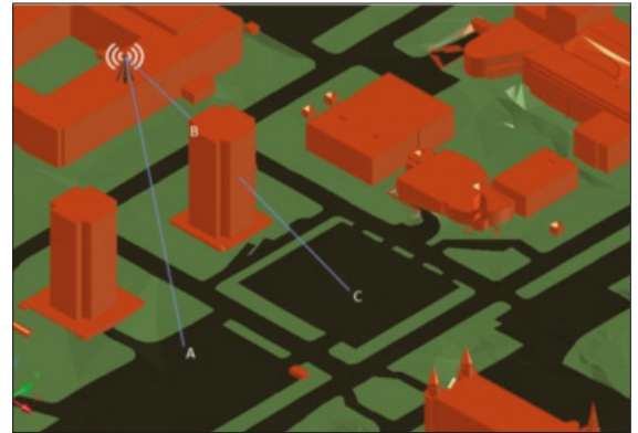
Direct visibility between an observer and a target, point A is visible while point C is invisible because its line-of-sight is concealed at point B. (See / Voir page 291)
