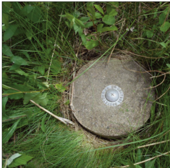
Figure 1: Geodetic control monument.
